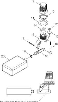
Note: The thinner tear-out distance of the W80B11P Float Arm should face upward.
